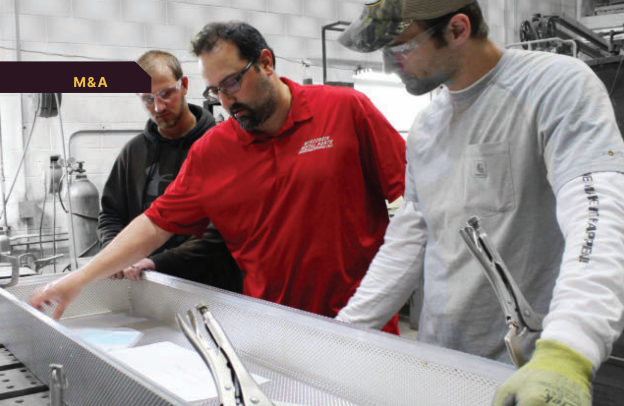
Technicians at SOLV Metals' Wisconsin Metal Parts inspect a perforated enclosure after forming. Images: SOLV Metals
