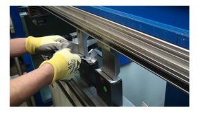
Tighter tolerances: Bending tolerances are another factor to consider. While a stamping die will typically hold tighter form tolerances and have better repeatability, newer CNC brake presses can be honed to hold bend tolerances as tight as .005" in some cases. Please see one of their most recent PDF's: What tolerances can WMPI hold for fabrication?
