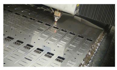
Technological advances in metal fabrication offer manufacturers many more options today that did not exist a decade ago. An emerging trend is to use a combination of fiber laser cutting and stamping die. Laser cutting can serve as a bridge to production while hard tooling is being built, thus shortening your lead time to market. Lasers can also be an economical way to work through prototyping and testing. https://www.wisconsinmetalparts.com/proj-clamp-prototype.html
